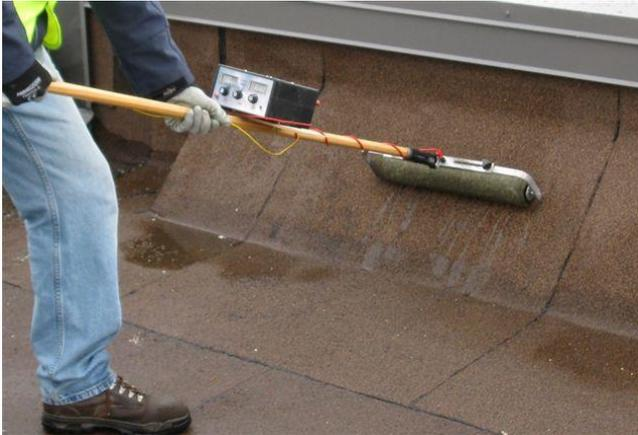
The moistened sensor is pressed against the surface area being tested. This action forces water onto the membrane surface and into any unsealed seam. At a breach location, a leakage current will flow from the ground connection to the breach location and returns to the receiver through the moisture sensor. The receiver will register a deflection on the signal level meter accompanied by an audible alert.
